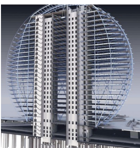
Figura 39 | Estrutura Aldar Headquarters . Render
