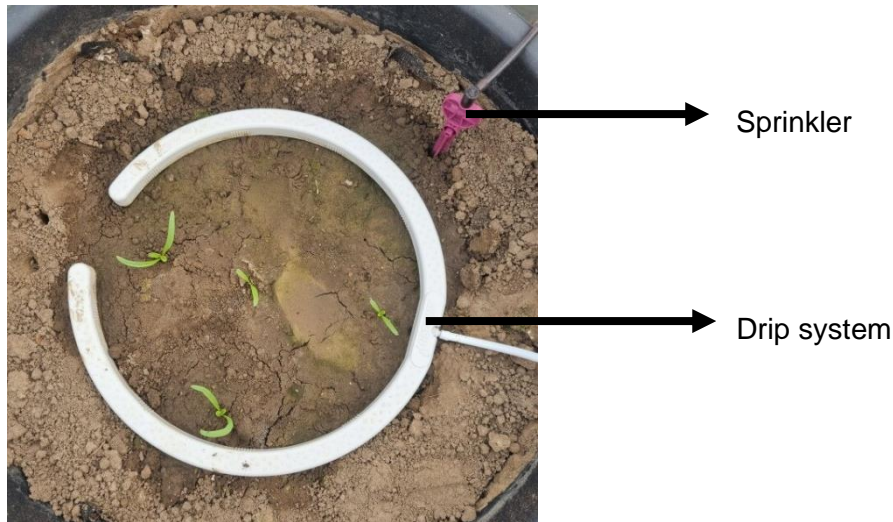
Figure 12: Pot irrigation scheme, where the purple stick is the sprinkler and the white ring the drip system
