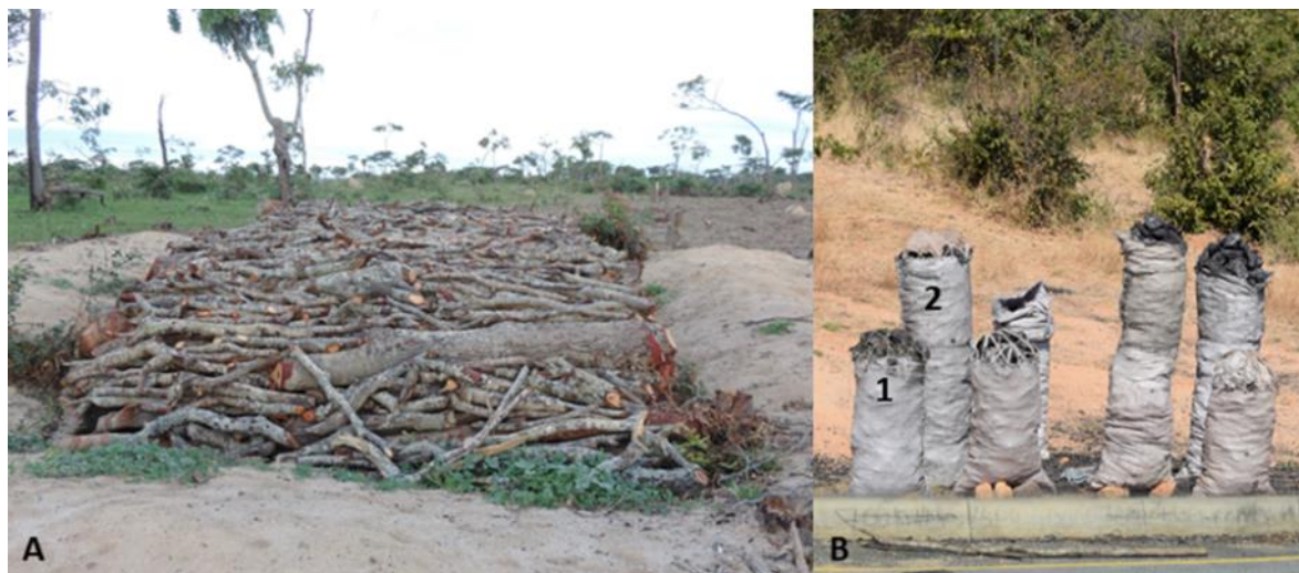
Fig. S1. A kiln dug into the ground before the carbonization process; B: the two main types of bags in which coal is usually packed and marketed: 1) ordinary bag; 2) large bag.
