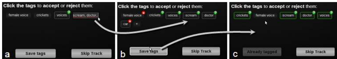
Figure 4.4: Labelling the audio excerpt: a) two labels suggested, one candidate for insertion (the one with the grey frame), and introducing new ones in a comma separated list; b) accepting (✓) and rejecting (×) tags; c) labelled audio with three tags introduced by the user, a suggested tag accepted and another suggestion ignored.
