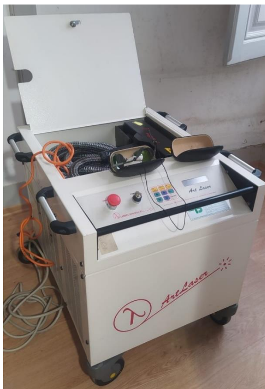
Figura 47 | Art Laser - Nd: Yag Q-Switch. © Débora Chaves
