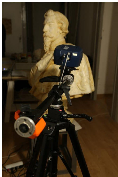
Figura 35 | XRF no busto D. Fernando II, © PSML, FBAUL, Débora Chaves.
