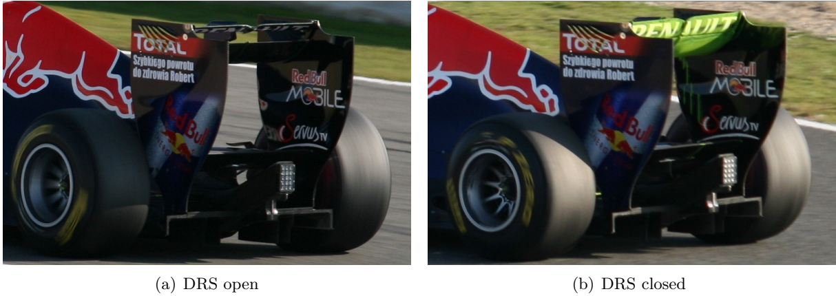
Figure 2.7: DRS mechanism of the Formula One Red Bull Racing's RB7 [11].
