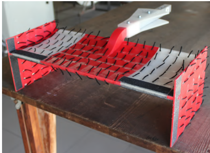
Figure 1.6: 3D printed model of a rear wing design studied in [6].
