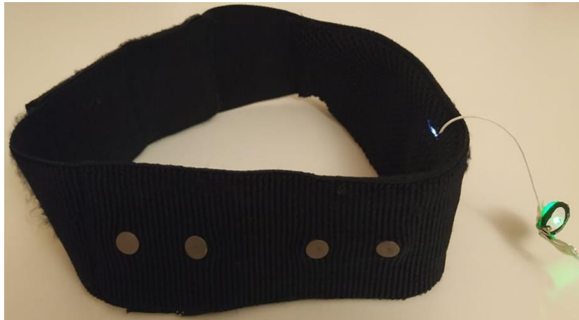
Figure 3.1 - Wearable EEG band used to collect the data with the two pairs of electrodes on the inside to positionate in the forehead of the patient, as well as the light sensor to track blood volume data in the form of a clip.
