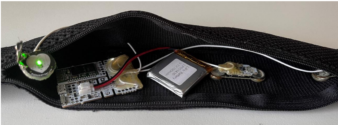
Figure 3.3 - Inside of the EEG wearable band with all the elements and the connections, these being micro-controller unit with the Bluetooth connector, as well as the two EEG units.
