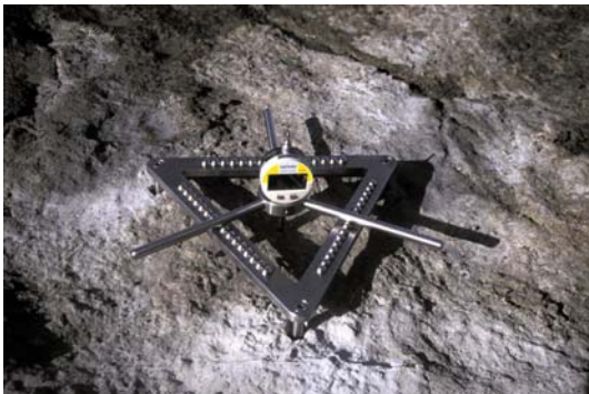
Figure 30. 1-TMEM installed in one of the studied areas; 2-Relative position of the 255 points measured by the TMEM.
