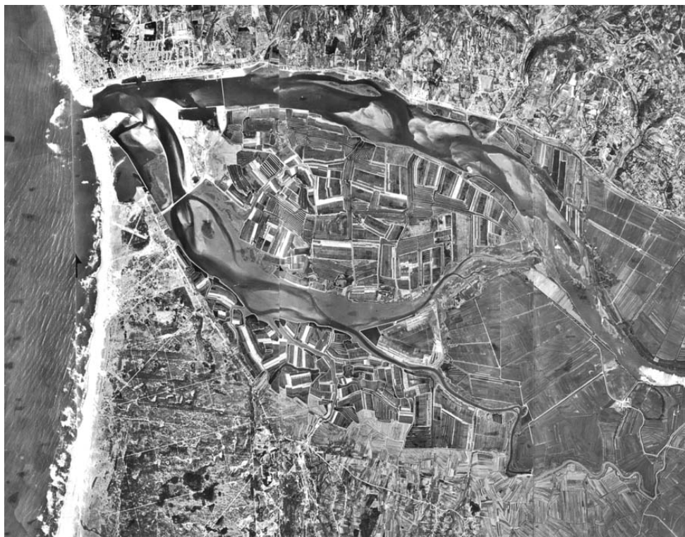
Figure 22. Mosaic of vertical aerial photos of the Mondego estuary (comprising the 9km downstream) in a spring low tide of 1947 (summer). The human interventions were reduced and limited to the mouth area. Notice the general silting of both estuarine branches.
