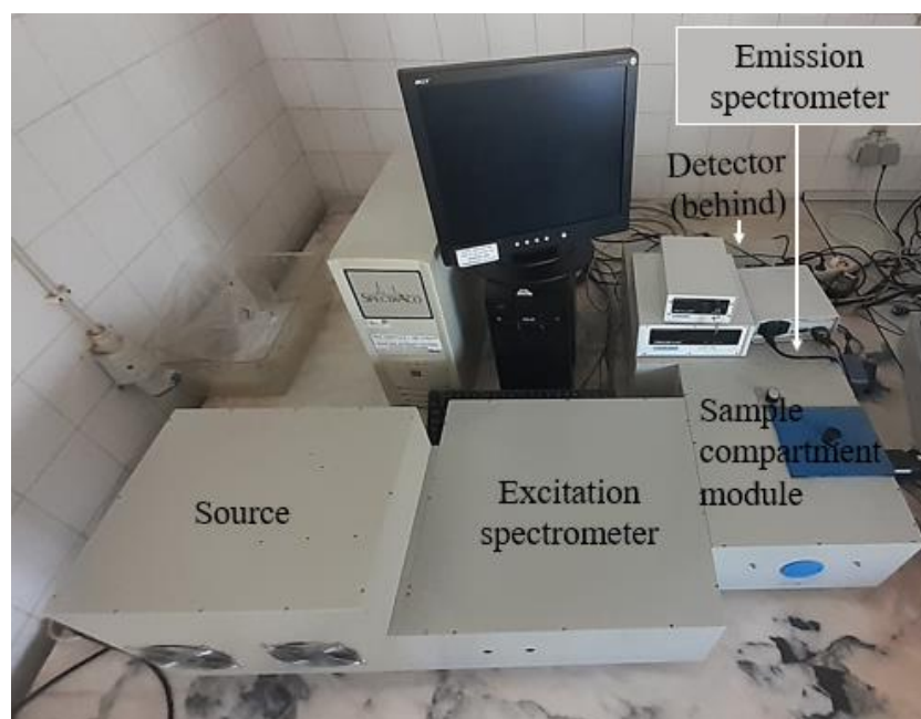
Figure 2.1. Fluorolog Model 3.22 Spectrofluorimeter from Horiba Jobin Yvon. This is the equipment used for the fluorescence spectroscopy measurements and the identification of each compartment.
