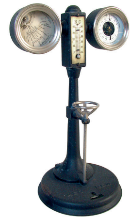
Figure 5 - BEW Model R Thermometer (1908). AEG. Peter Behrens. Metal, Thermometer. This very rare object made by AEG was amongst the first designed by Behrens for the brand. Rare for its inclusion of the initials AEG-BEW – the latter referring to the AEG subsidiary Berliner Elektrizitätswerke – this desk item comprises a thermometer, hygrometer, barometer, and calendar. The hygrometer uses a dial that predates Behrens and displays Jugendstil influences, perhaps designed by Otto Eckmann, one of the brand's first designers. All of the measuring instruments, as well as the frame, clearly show the Behrens style.
