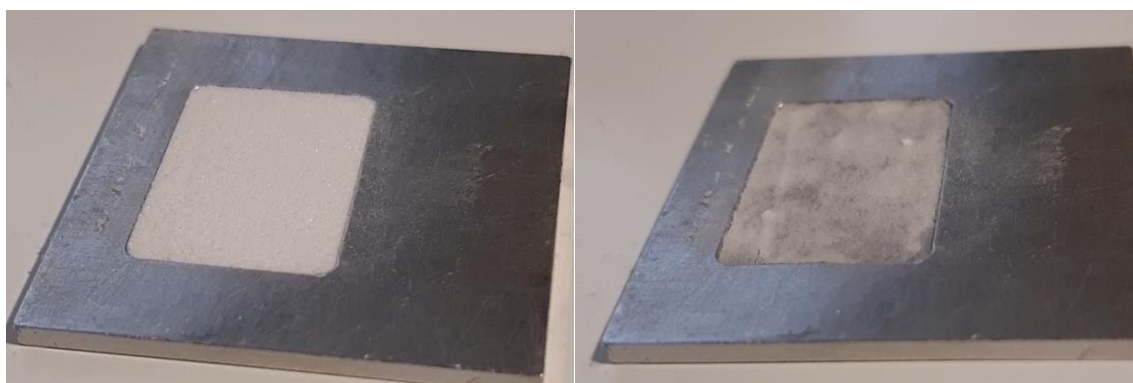
Figure 2.3. Morphology of the PM sample before (left) and after (right) heating to 423 K.
