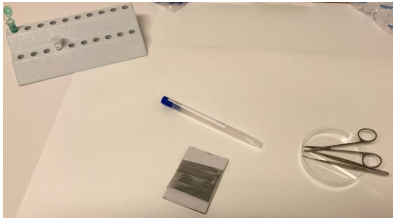
Figure 3.3: Sampling procedure of experiment 3, transfer and persistence by handling of tape. In this figure we can see the “drug wrap” (cardboard wrapped with tape) and the equipment used for sampling in experiment 3 (tweezer, scissors, swab and the eppendorf tube).
