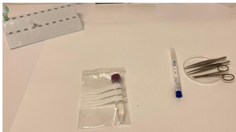
Figure 3.2: Sampling procedure of experiment 2, indirect transfer. In this figure we can see a zip lock bag containing a tube filled with water (the tube is discarded) and the equipment used for sampling in experiment 2 (tweezers, scissors, swab and the eppendorf tube).
