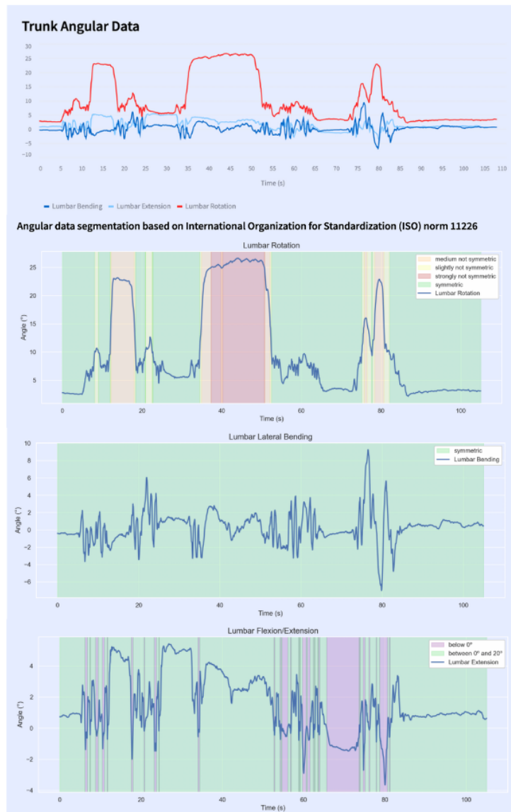
Figure 5.6: Dashboard's section for data visualisation. The data refers to the trunk and the segmentation presented is based on angular limits ("Posture Segment").
