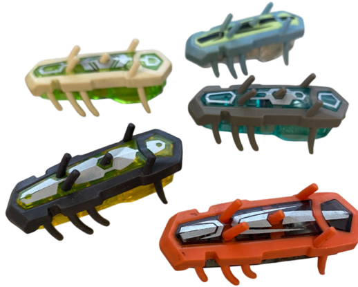
Figure 5.1: HEXBUG robots used as macroscopic active particles, with approximate dimensions of 40 \times 15 \times 20 mm and mass 7.2 g. Each device self-propels via internal vibration and undergoes random reorientation through frictional interactions.
