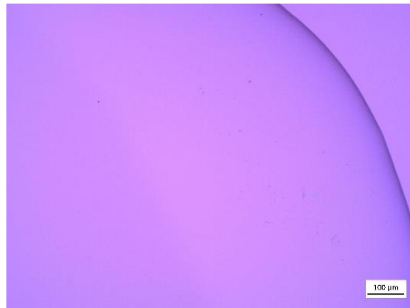
Figure 4.2. Microscopical observation of the peripheral region of 5% DM (w/w) loaded PLGA films using methanol as a co-solvent, dried under the hood overnight.
