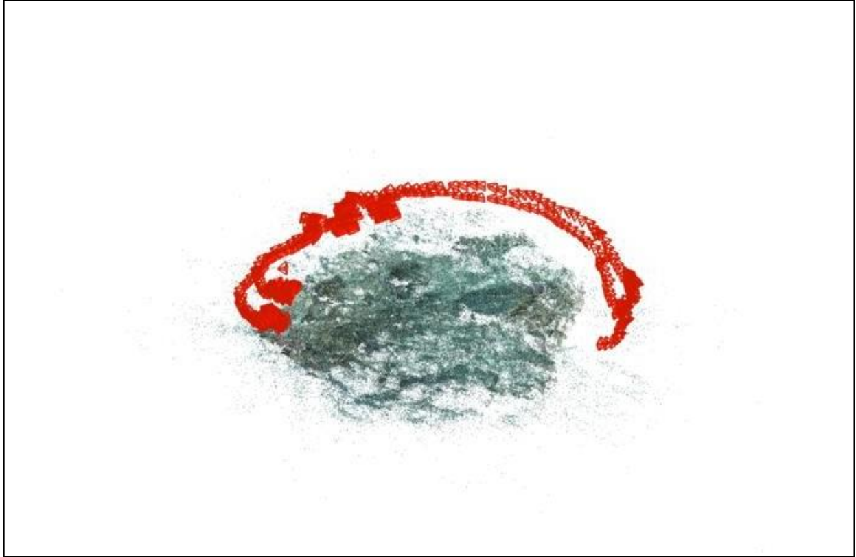
Supplemental Figure 4. Dense cloud point and camera positions outputed from colmap after image sampling and scene reconstructions (animation by ©Fritz Francisco).
