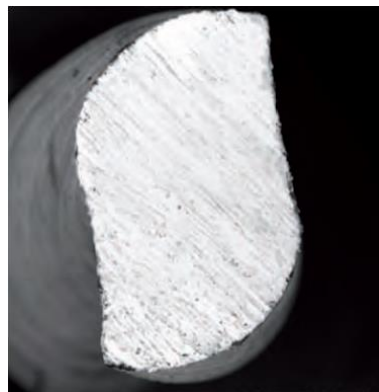
Figure 6 – S-shaped cross section of Reciproc® files (VDW, Munich, Germany).
