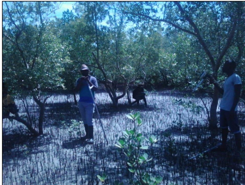
Figure 18 - Measuring tree height with a bamboo stick.
