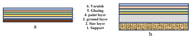
Fig. 1 Representation of the painting system of a painting on copper (a) and a painting on canvas (b)
