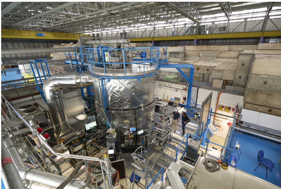
Figure 1.1: The CLOUD chamber, the central component of the experiment at CERN. The stainless-steel sphere, with a volume of 26 cubic meters, serves as a precisely controlled environment for studying atmospheric nucleation. The intricate network of pipes, cables, and external instruments connected to the chamber's many access ports highlights the complexity of the experimental setup required to control and measure a wide range of atmospheric parameters.
