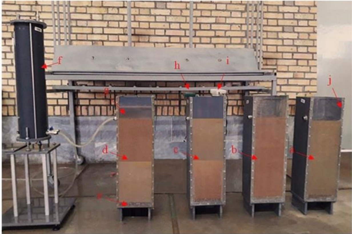
FIGURE 2 The set-up of experiments: (a) the column of sandy loam, (b) the column of clay loam, (c) the column of two-layered soil (sandy loam (up) and clay loam (down)), (d) the column of two-layered soil (clay loam (up) and sandy loam (down)), (e) filter, (f) Mariotte bottle, (g) water head, (h) watermark and (i) wet sensor and (j) soil container
