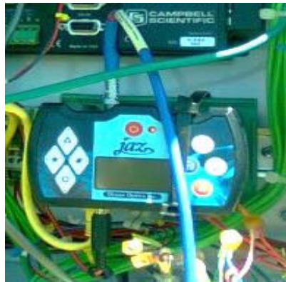
Figure 26 – Jaz spectrometer inside the instruments cabinet on the chassis. The optical fiber (blue) that attaches to the device is also visible.
