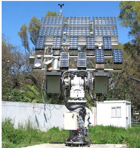
Figure 22 – Overview of the two-axis tracking platform with several mounted modules. The PC cabinet is also visible further on the back.
