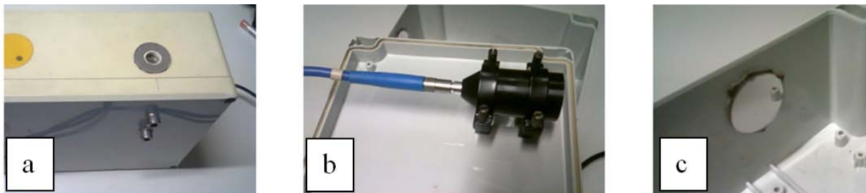
Figure 27 – Spectrometer fibre box detail: a) quartz window, b) optical fibre connected to the circular collimator and c) reflective neutral density filter.
