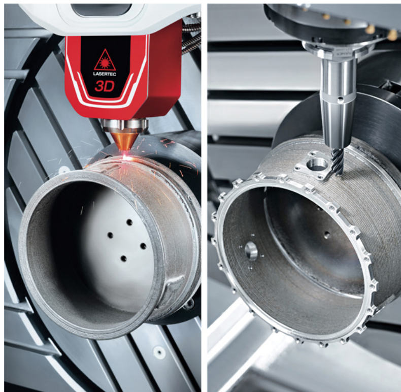
Figure 32: Example of building a part with a hybrid fabrication method, combining laser deposition AM and subtractive fabrication (CNC milling) done on a DMG Mori LASERTEC 65 3D hybrid manufacturing system. (Waterman, 2016)
