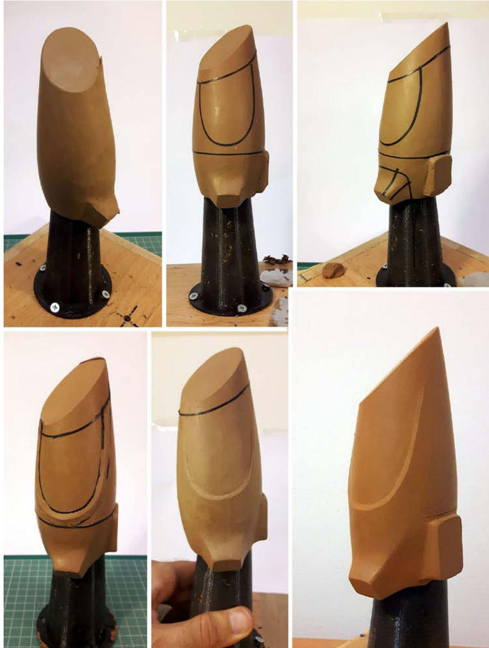
Figure 74:Progress photos of the clay model's surface refinement manually
