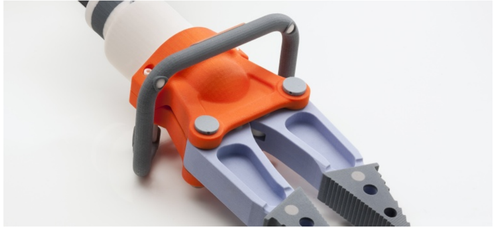
Figure 30: Image of a PP fabricated with Color Jet Printing (CJP) (Addema, n/d)
