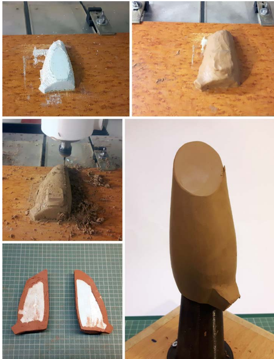
Figure 73: Prototyping process using RP CNC milling machine and automotive grade oil-based clay from Kolb-Technology.
