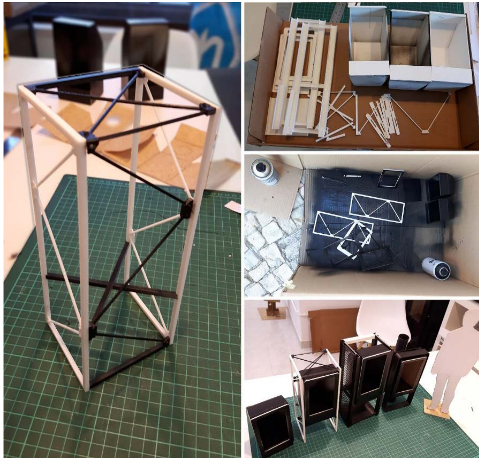
Figure 51: Fabrication process of presentation models with a combination of traditional modelmaking tools and AM, rapid prototyping technology.
