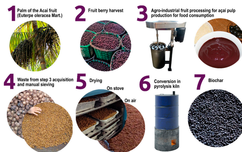
Figure 1. Scheme of biochar production using acai berry fruit waste as raw material, from palm, harvest, agro-industrial processing, waste generation, sieving, drying, and conversion.
