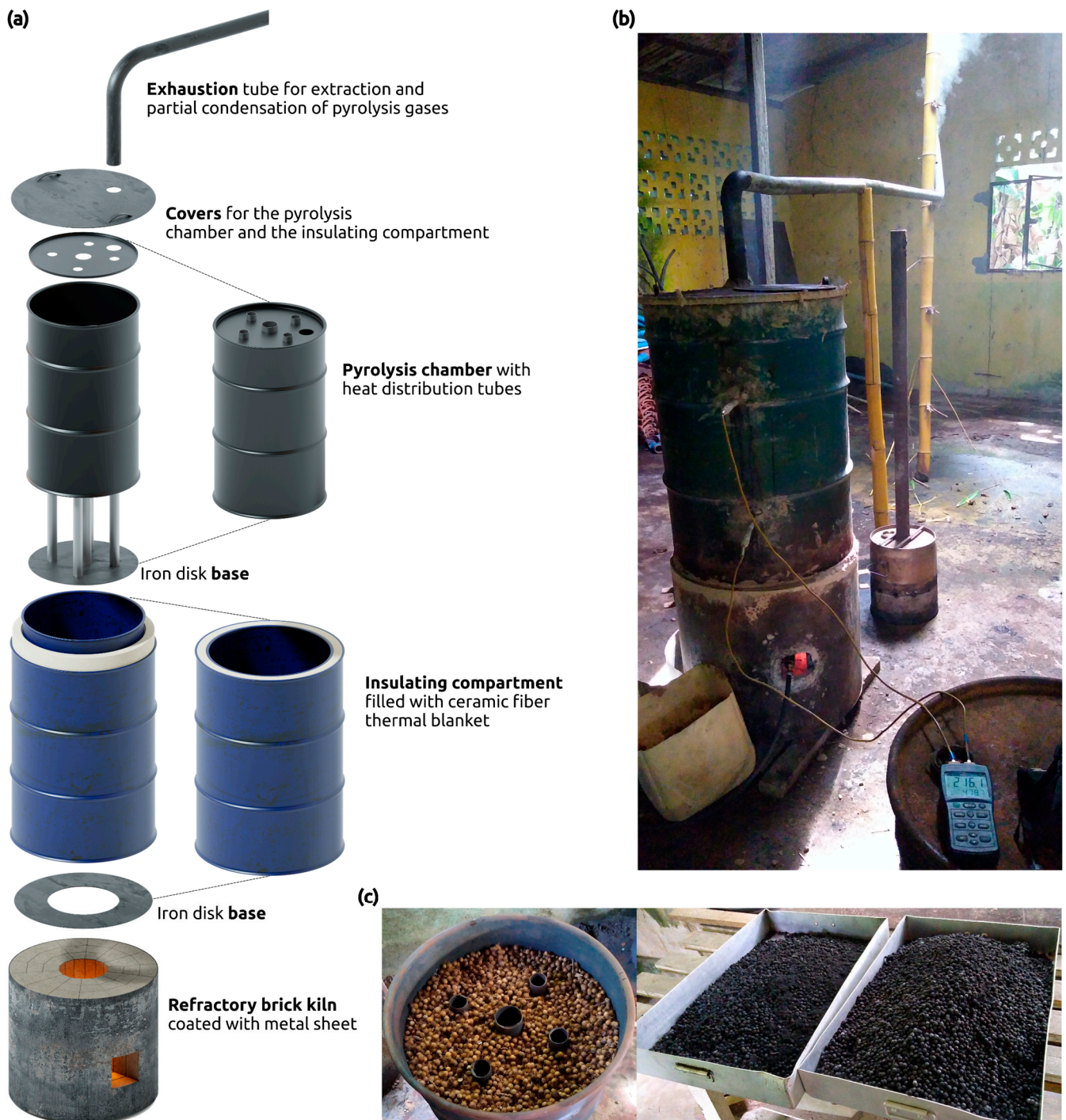
Figure 2. (a) Three-dimensional schematic of the construction of the low-cost mobile pyrolysis kiln; (b) photograph of the kiln in operation; and (c) photograph pyrolysis chamber fuelled with acai berry biomass and the produced biochar.
