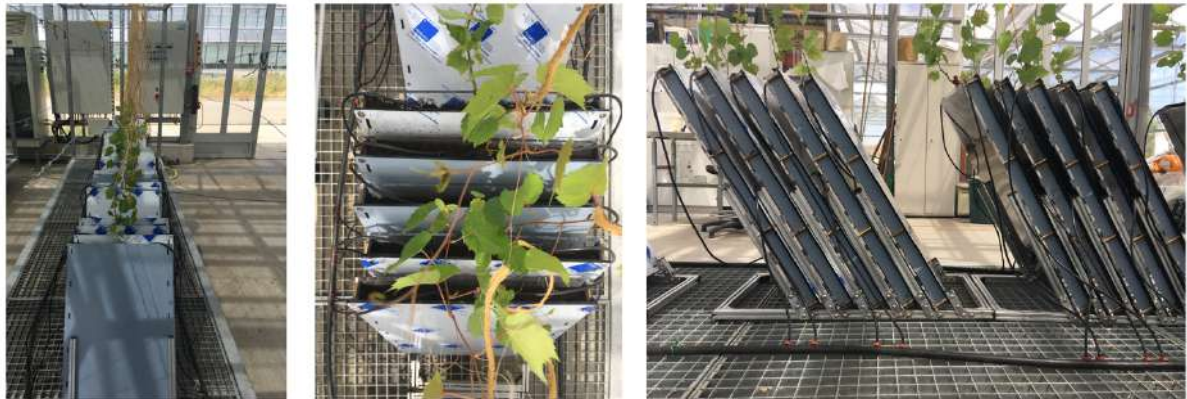
Figure 14 For the implementation of the rhizobox experiment, 24 rhizoboxes were filled with substrate and populated with 3309 C cuttings. Two 25 l jerrycans supplied nutrient solutions by pump support. One main hose per jerrycan branched into two irrigation hoses per rhizobox. Inclined positioning of the boxes promotes root growth onto the transparent back panel of the boxes. Each last box in one block was sheeted to prevent excess light exposure.
