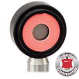
Figure 3.22: Image of the compact photodiode power head with silicon detector: S120C from Thorlabs[28].
