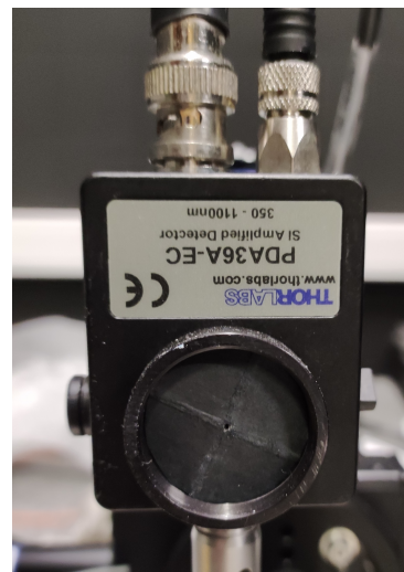
Figure 3.15: Photograph of the detector A with an active area of A = 0,79mm^2 , created using a diaphragm.
