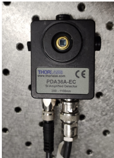
Figure 3.14: Photograph of the detector B with an active area of A = 13mm^2 .
