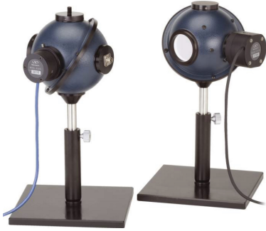
Figure 1.1: Image of an example of a small integrating sphere is this model 819D-SL-2 from Newport . An IS with 3 ports, a diameter of 5\text{cm} (PTFE).[4]
