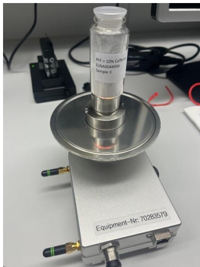
Figure 16: Example of off-line sample measurement with NIR spectrometer.
