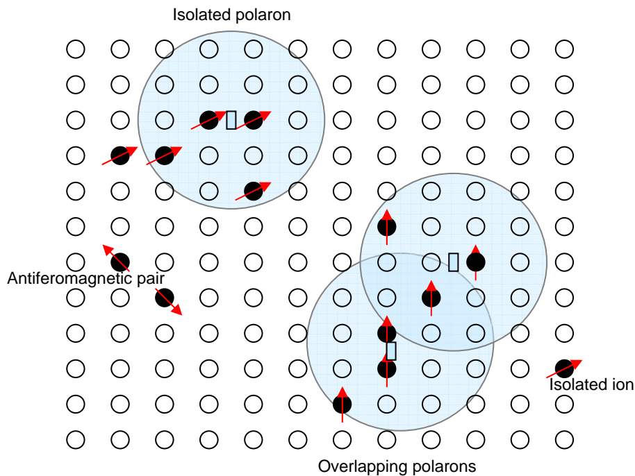
Figure 2.7 Polaron percolation model as illustrated by Coey et al. 23 .
