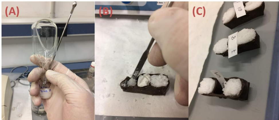
Figure. 3.1. Scaffolds sequence preparation: (A) is the PDLLA dissolution with DMC and the mixing of BG, followed by the porogen (salt) addition; (B) corresponds to the final mixture being transferred to a flexible square silicon mold; (C) shows the prepared samples in a vacuum chamber to eliminate the solvent.
