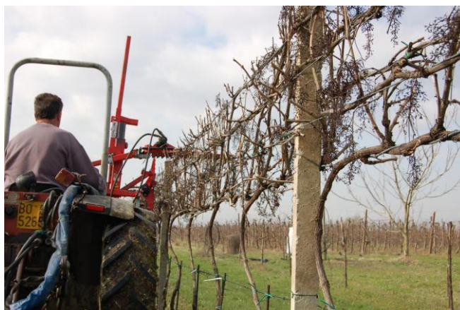
Figure 2 Mechanical pruning on a semi-minimal pruned hedge (SMPH) system (extracted from Intrieri et al., 2011).
