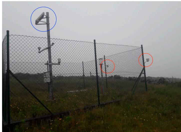
Figure 3. Strategic placement of the IoT sensors used for validation: NVX_R712_00137A1000015794 and NVX_R712_00137A1000015795 (red), and the reference meteorological IPMA station 11217372 (blue).
