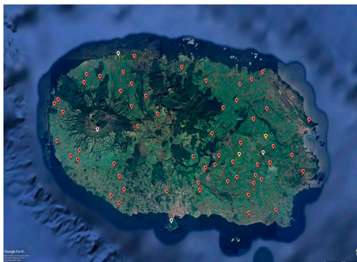
Figure 2. Deployed IoT network configuration. R712 type (red), DL-SHT35 type (yellow), gateways (white). The illustration was developed in the Google Earth Pro app.
