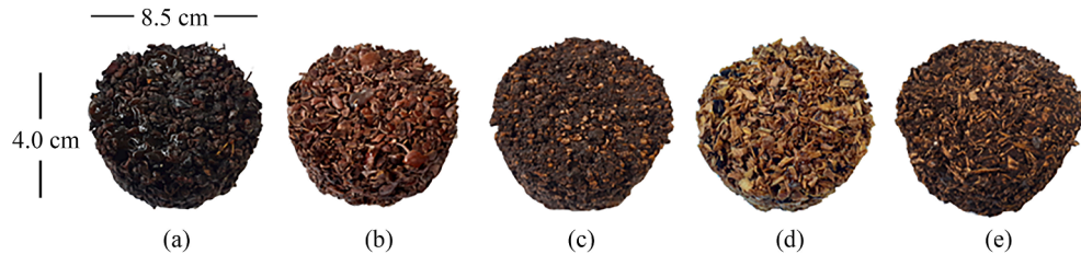
Fig. 3. Samples B – sodium silicate solution: (a) grape press waste (BG); (b) hazelnut shells (BH); (c) olive press waste (BO); (d) wood chips (BW); (e) wood chips and spent coffee grounds (BWc).
