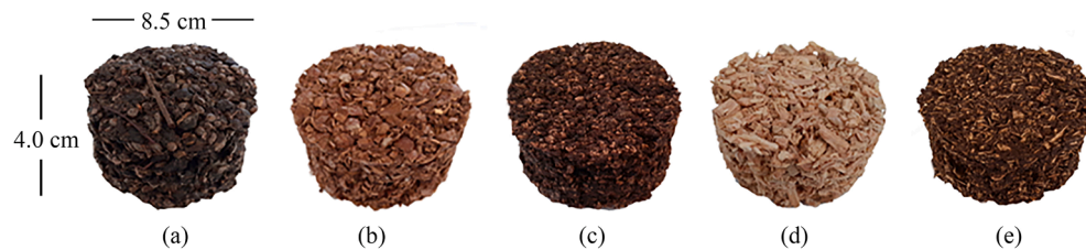
Fig. 4. Samples C – starch-based natural glue: (a) grape press waste (CG); (b) hazelnut shells (CH); (c) olive press waste (CO); (d) wood chips (CW); (e) wood chips and spent coffee grounds (CWc).
