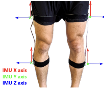
Figure 3.7: Placement of the IMUs on the subject's legs using velcro straps.
