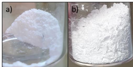
Figure A.1 – a) MOF-5-S1 and b) MOF-5-S2 obtained powders via solvothermal synthesis.
