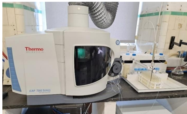
Figura 21 - ICP (Thermo Scientific iCAP 7000 Series ICP- OES)
