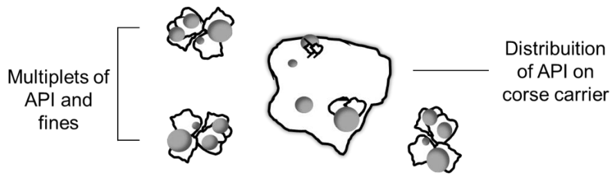
Figure 2.24 – Schematic representation of the hypothesis of formation of agglomerates with drug and fine excipient particles (multiplets) during blending.
