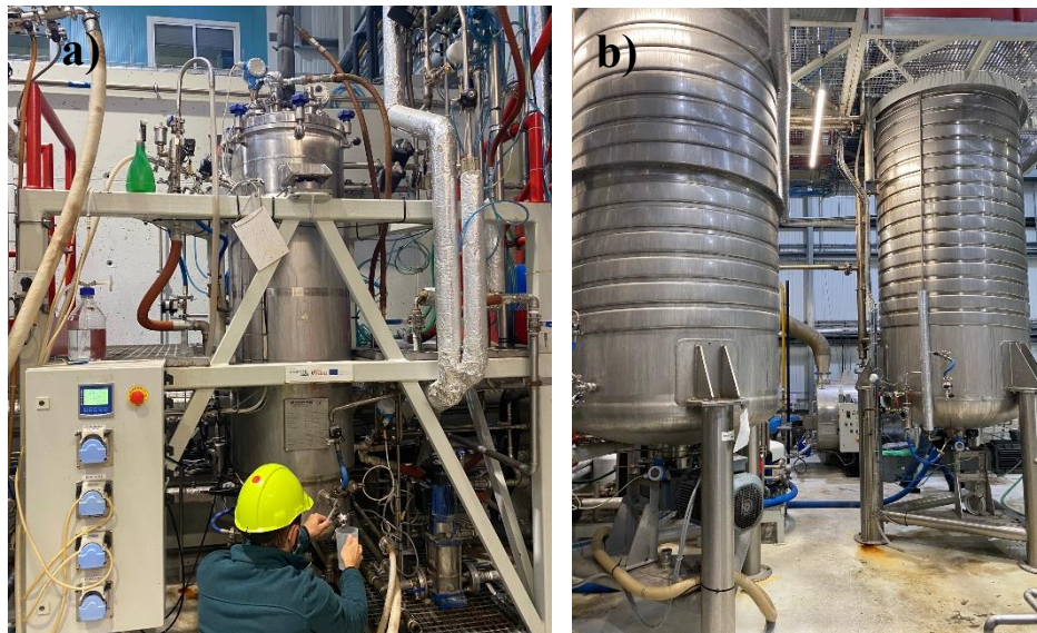
Figure 3.2: Heterotrophic growth, an example of a) 200 L fermentation reactor and b) 5000L fermentation reactors. Photos taken at Allmicroalgae company.
