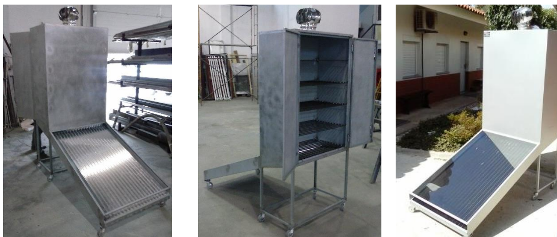
Figure 3.2 Illustrative aspect of the “DNB” solar dryer while under the construction process at SISELM, Lda.
