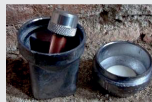
Fig. 2 Dosimeter capsule inside a lead box.
