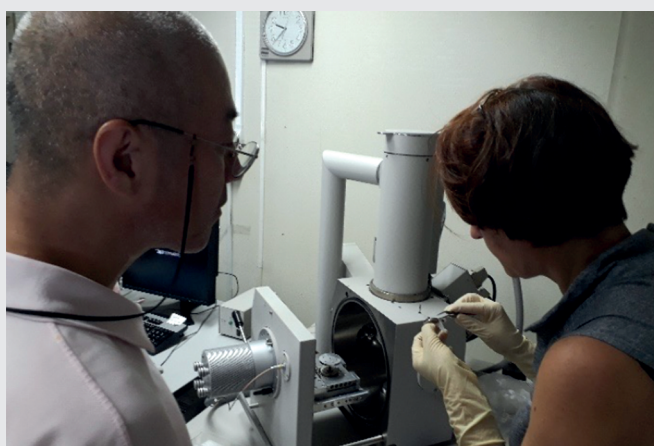
Fig. 1 Japanese and European researchers analyzing glass beads by SEM (left) and FORS (right).
