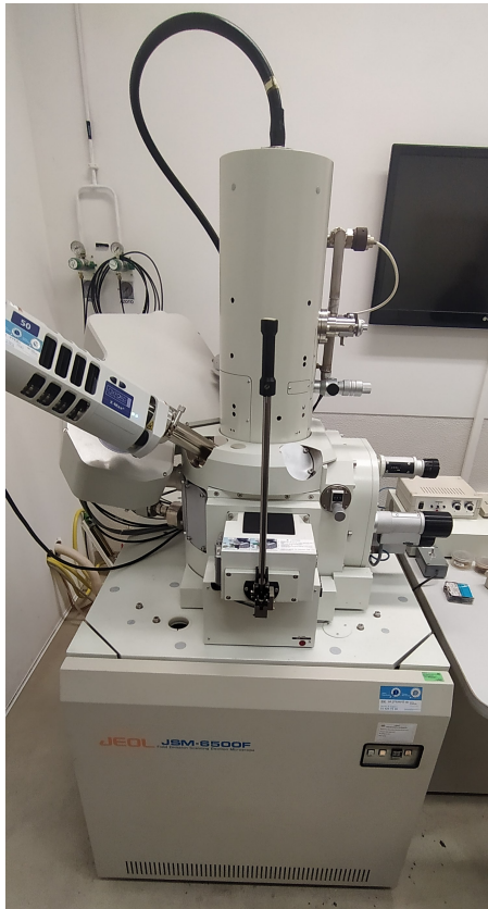
Figure C.10: SEM microscope JEOL JSM-6500F and detail from the EDS Oxford Instruments X-Max N .
