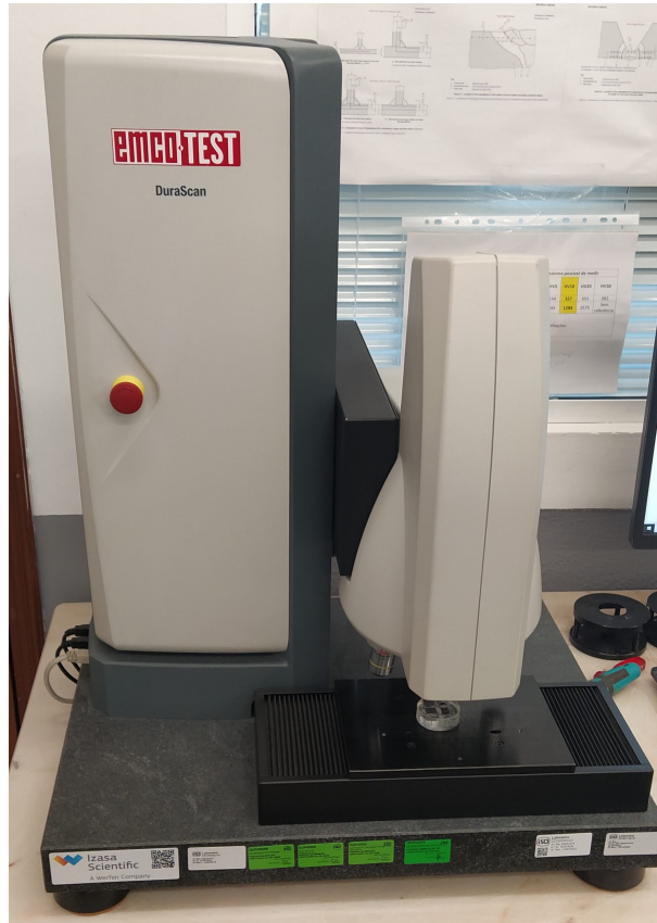
Figure C.14: Hardness measuring machine EMCOTEST DuraScan 70 G5 . Possible to measure Hardness Vickers and Brinell.
