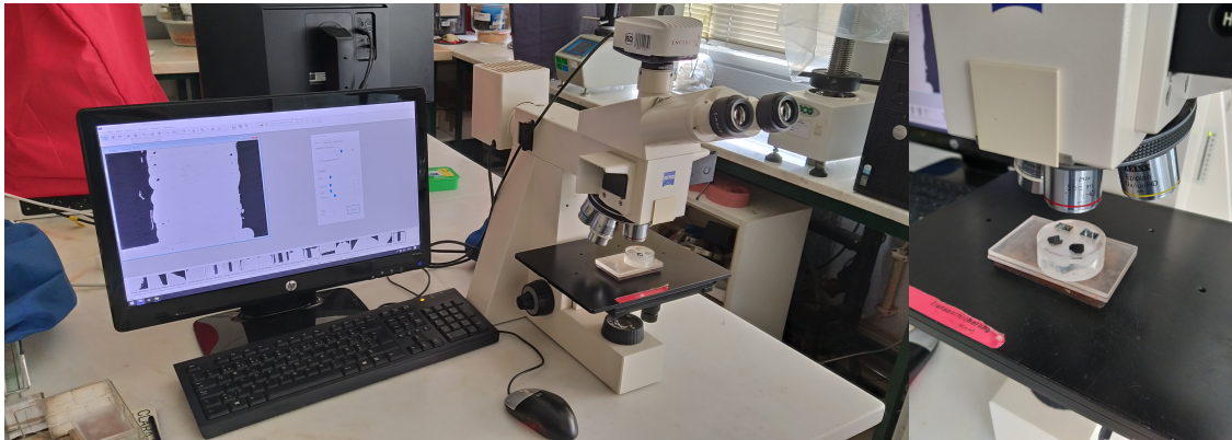
Figure C.6: Setup with optical microscope ZEISS AxioTech 100 and detail from the analysis area with a mounted sample being observed.
