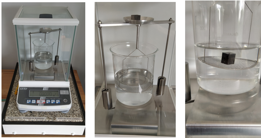
Figure C.9: Balance used for density measurements, Kern ABS 220-4N (a), mass measurement of one sample in air (b) and inside water (c), using the same balance.
