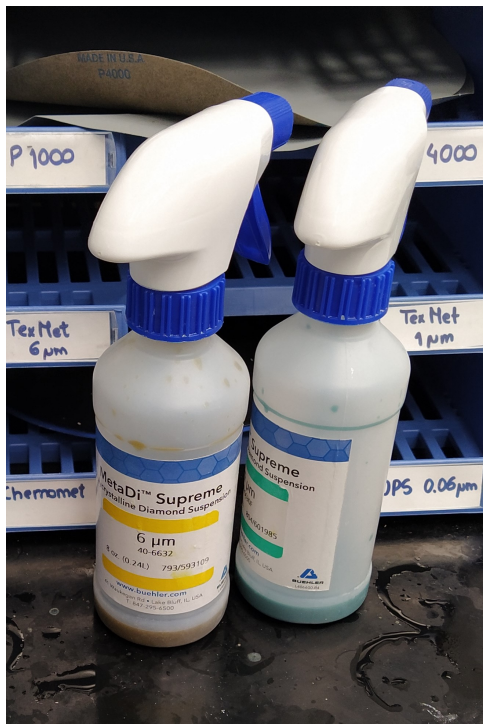
Figure C.5: MetaDi Supreme Crystalline Diamond Suspension for 6 and 1 \mu\text{m} mats (left) and MasterMet Colloidal Silica Polishing Suspension (right), both from Buehler .
