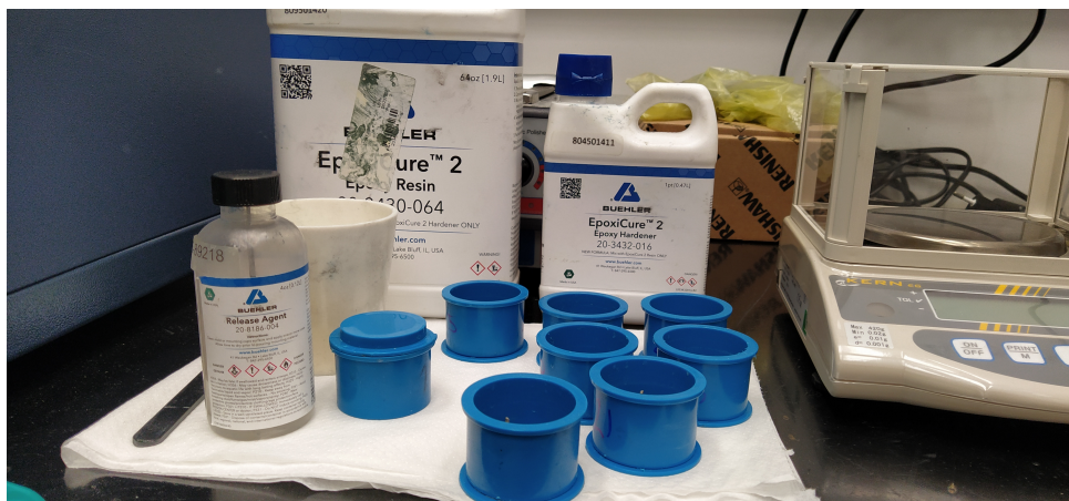
Figure C.3: Equipment used for making epoxy samples. The three liquids observed are the Buehler Epoxy Resin, Epoxy Hardener, and Epoxy Release Agent, respectively from the bigger to the smaller recipient. At the right is shown the balance used to weight the liquids in the right proportions. In blue are shown the cups to fill with the epoxy mixture.
