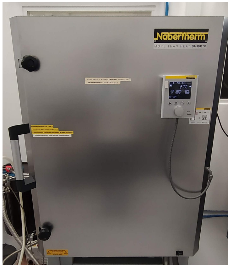
Figure C.7: Chamber furnace LH 30/14 from Nabertherm . Could heat up to 1400°C.
