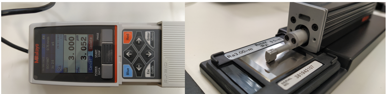
Figure C.13: Mitutoyo SJ-210 portable surface roughness tester and detail from the cantilever of the machine doing a calibration process.
