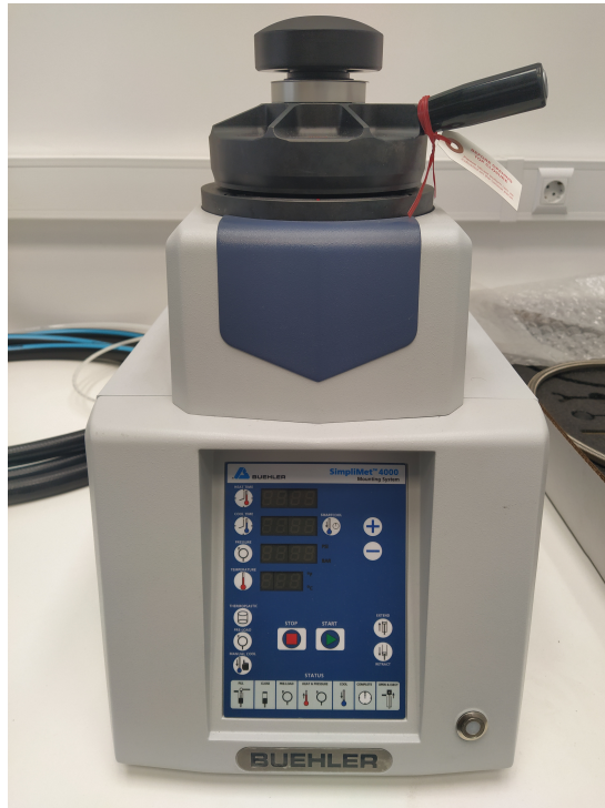
Figure C.12: Mounting machine SimpliMet™ 4000 Compression Mounting System from Buehler .
