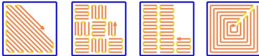
Figure 1.10: Schematic of several scanning strategies commonly used in PBF-LB. Respectively from left to right, Meander, Chessboard, Stripe and Spiral, [27].
