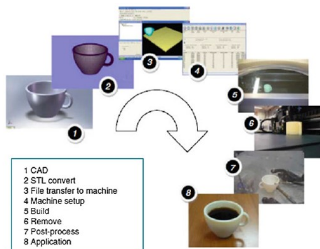
Figure 1.1: Steps of an AM process, starting from the 3D design until the application, [5].
