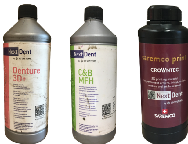
Figure 1- Photographs of the NextDent resins used in specimen production: Denture 3D+® (colour Translucent Pink, lot number WY213N01, expiration date 20.05.2022), C&B MFH® (colour N1, lot number EX433N03, expiration date 27.10.2023) and Crowntec® (colour A2, lot number E276, expiration date 03.2025), in order.
