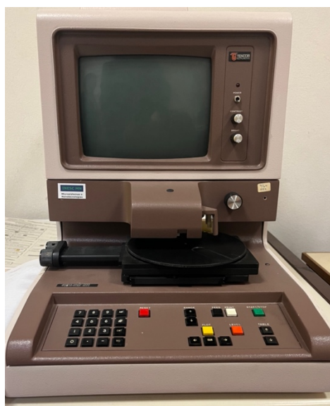
Figure 12 – Photograph of contact profilometer used Tencor® Alpha-step 200 Profilometer, available at INESC – MN.
