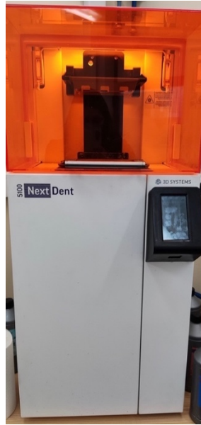
Figure 2 – Photograph of NextDent 5100® printer used in specimen production for groups ND, NC and NT.
