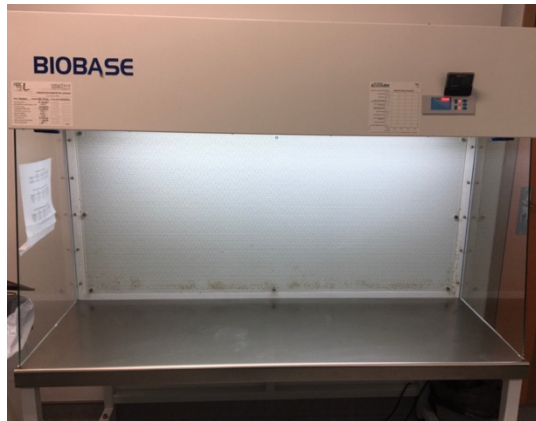
Figure 9 - Photograph of horizontal laminar flow chamber used during cell culture.
