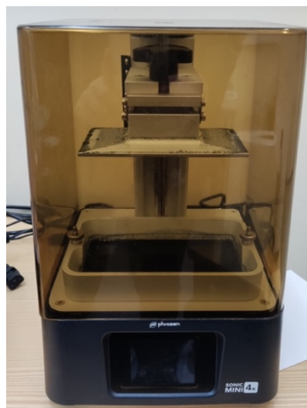
Figure 3 – Photograph of Phrozen Sonic Mini 4K® printer used in specimen production for groups PD, PC and PT.
