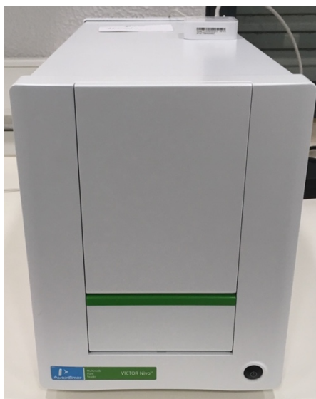
Figure 11 - Photograph of multimode microplate reader used during biocompatibility and interleukin essays.
