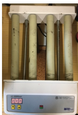
Figure 5 - Photograph of NextDent LC-3DMixer® roller bench used in sample production.
