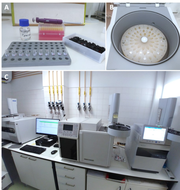
Figure 3.39 – Steps before the gas chromatography. A – Addition of toluene using a micropipette; B – Placement of the different vials in the rotary evaporator; C – Placement of the vials in the gas chromatograph carousel.
