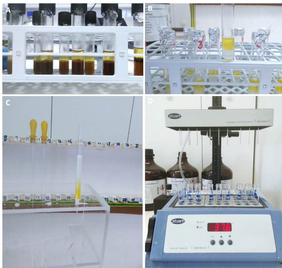
Figure 3.38 – Major steps in the APO fraction 'Clean-up' process. A – TLE saponification process; B – Upper phase separation after with \text{H}_2\text{O} milli-Q; C – Silica microcolumn separation eluted with HEX; D – Apo clean drying under a \text{N}_2 flow.
