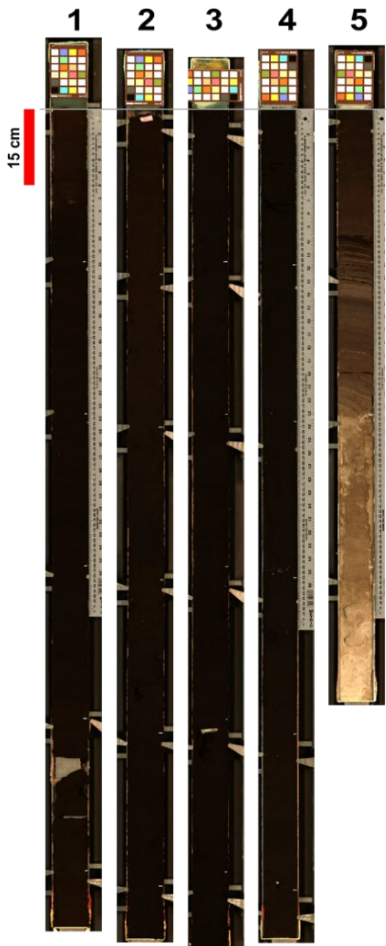
Figure A.56 – Half of the ‘PEX 19’ sediment cores in a color scan image with +25% luminosity. Total length: 8.43 m in length; width: 90 mm. The numbers identify the section number (1 – 5, from left to the right).
