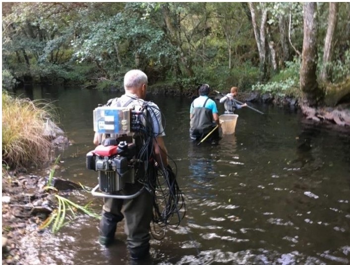
Figure 2.10 Sampling of fish using electrofishing.
