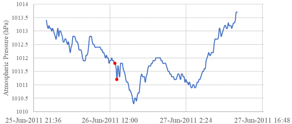
Figure 4.19. Atmospheric pressure from Peniche station. The sample interval is 10 minutes. The red dots identify the more significant jumps in pressure.
