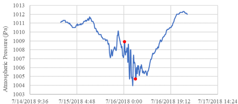
Figure 4.29. Atmospheric pressure from Ciutadella de Menorca station. The sample interval is 10 minutes. The red dots identify the time interval with more significant “jumps” in pressure.
