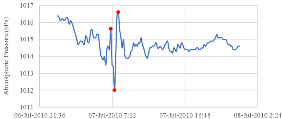
Figure 4.12. Atmospheric pressure from Peniche station. The sample interval is 10 minutes. The red dots identify the more significant jumps in pressure.
