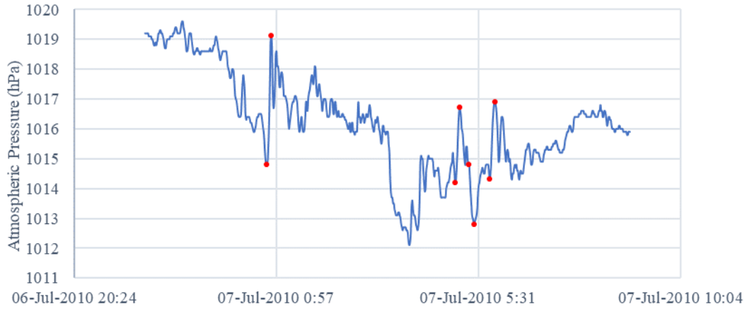
Figure 4.8. Atmospheric pressure from Sines station. The sample interval is 1 minute. The red dots identify the four more significant “jumps” in pressure.
