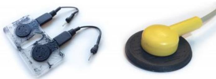
Figure 1.8: G. Wolterink, R. Sanders, and G. Krijnen 3D-printed sEMG sensor [44]
