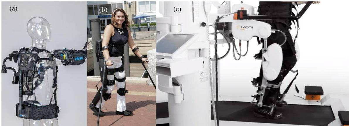
Figure 1.1: Examples of the several types of exoskeletons (a) EksoVest [5]; (b) ReWalk exoskeleton [6] ; (c) Lokomat [12]
