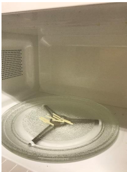
Figure 6: Microwave post-polymerization group (mw1). Specimens were directly placed in a microwave at 750 W for 1 minute;
