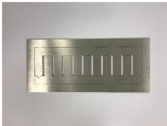
Figure 2: Stainless-steel mold used to fabricate the specimens.
