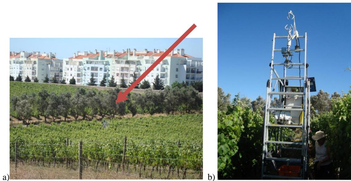
**Fig.III. 26: Instrumental eddy covariance measurements (EC) in Vineyard field experiment – Quinta do Marquês, Oeiras. a) EC localisation on the parcel. b) the sensors and the metal observation tower at the height of 2.5 m**
