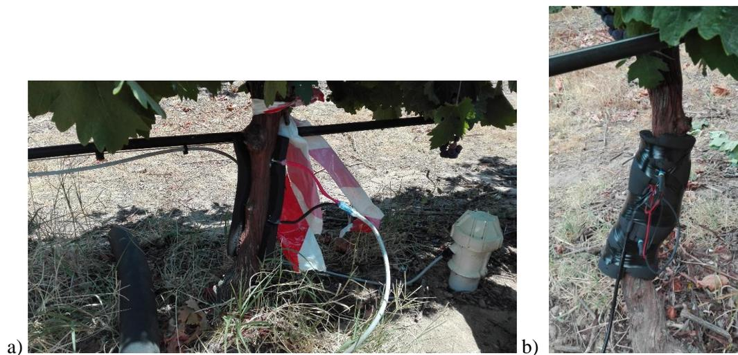
**Fig.III. 23:** The installation of sap flow sensors on the vineyard -Adega Catapereiro: a) modified *Granier* sensor; b) Conventional *Granier* sensor.
