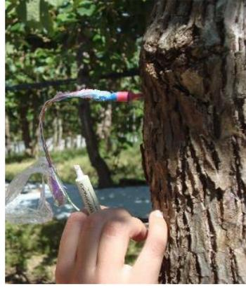
**Fig.III. 22:** The installation of modified *Granier* sap flow sensors on Kiwi plants in Briteiros (Guimarães, Portugal).
