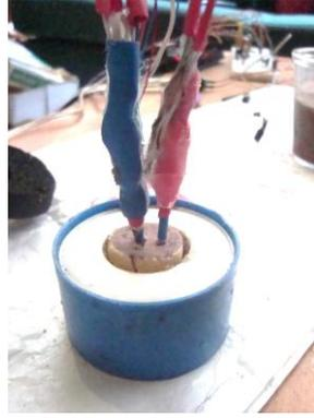
Fig.VI. 10: The heater sensors ( $G2J_{\text{heat}}[^\circ\text{C}]$ ) and referential sensor ( $G2J_{\text{no\_heat}}[^\circ\text{C}]$ ) inserted into a tube filled with cork
