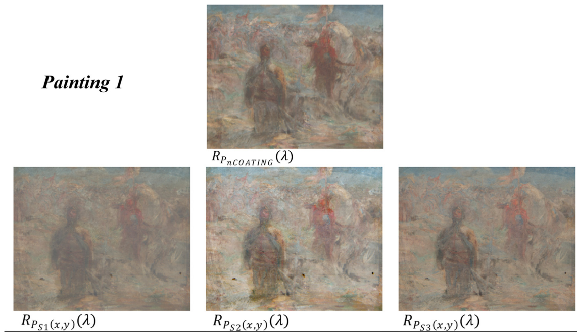
Fig. 8. sRGB renderings of the reflectance data retrieved from the original Painting 1 without the coating ( R_{P_{nCOATING}}(\lambda) ) and the three simulations of the virtual removal of the coating ( R_{P_{S1}(x,y)}(\lambda) , R_{P_{S2}(x,y)}(\lambda) , and R_{P_{S3}(x,y)}(\lambda) ) for simulation methods 1, 2 and 3, respectively. These images do not represent true colors and are intended only as visual representations of the simulation results. Quantifications of the simulation results are represented in Table 2 and Table 3.
